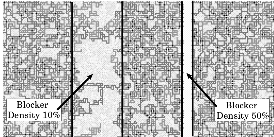
Fig. 6. The use of “walls” to modularize neural circuits in the new CAM-Brain model. The density of blocker instructions on the chromosome determines the probability of trail-growth through a wall and hence the penetrability of the wall.
